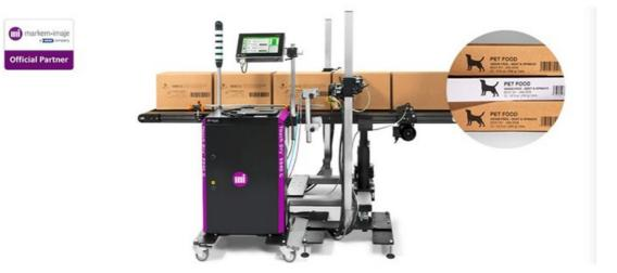
The 5940 G features Markem-Imaje's proprietary Touch Dry inks that instantly dry on contact. This not only increases readability but also offers more reliable traceability. And, unlike liquid inks, Touch Dry inks are ideal for secondary packaging because they don't lose resolution by spreading along corrugated fibres. The inks, which are available in a variety of colours, are VOC-free, safe to handle, and support sustainability.
