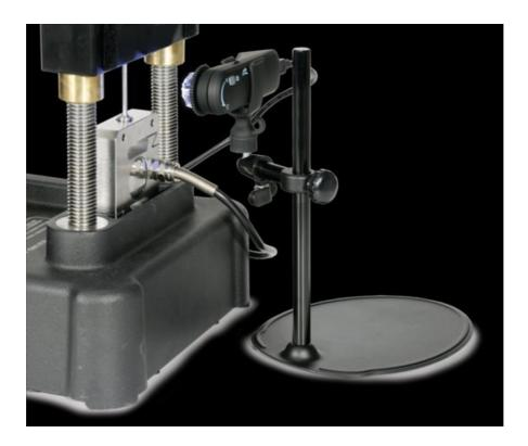
This Microscope Camera includes a stand, built in adjustable LED lighting, and has a 60x Optical Zoom. You can see even the tiniest changes during an experiment (as pictured for stress and strain) or else use it as a working microscope for Life Science activities.
