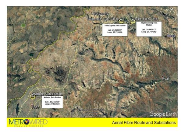
The aerial fibre route is built over mountain and rugged terrain using powerlines across three substations in the districts of Mabote, Saint Agnes and Teyateyaneng.
