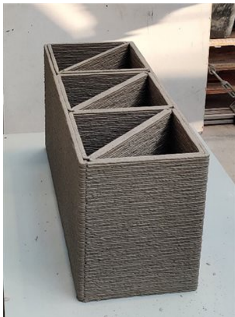
A building envelope prefabricated using the 3D printing process. Mehdi Chougan, author provided
